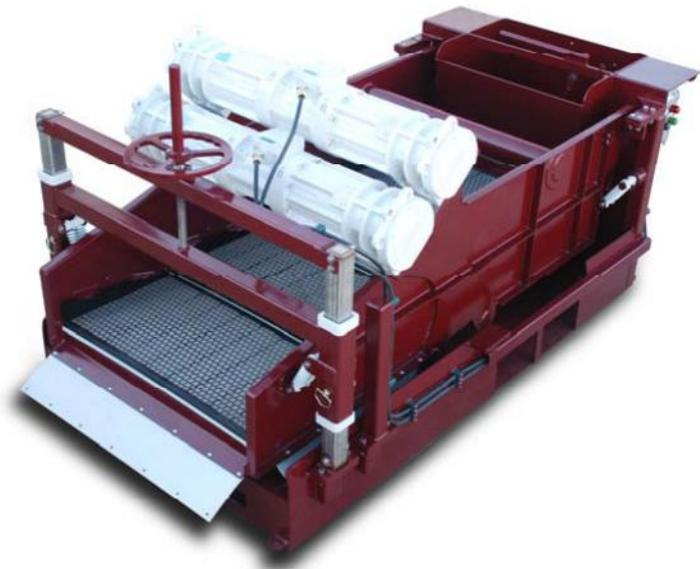
Scomi Equipment Inc offers a comprehensive range of Solids control equipment for oilfield applications. The Scomi Equipment Inc line of high performance shakers are specifically designed and engineered to efficiently and reliably separate solids from drilling mud.
