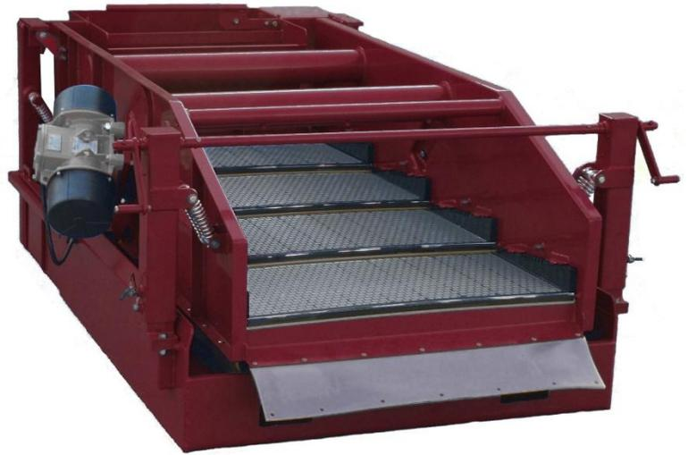
Scomi Equipment Inc offers a comprehensive range of Solids control equipment for oilfield applications. The Scomi Equipment Inc line of high performance shakers are specifically designed and engineered to efficiently and reliably separate solids from drilling mud.
